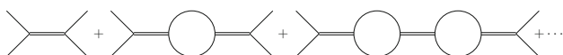
Fig. 1 Feynman diagrams for the two-particle scattering. The double lines denote the bare state
