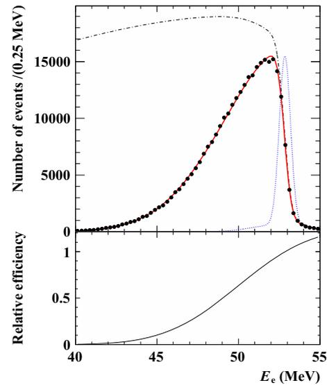
**Fig. 2** Michel positron spectrum (*top*). The *dots* are data and the *red-solid line* is the best-fit function. The *blue-dotted line* shows the detector resolution and the *dot-dashed line* shows the theoretical Michel spectrum, folded with the detector resolution. The *bottom plot* shows the energy dependence of the acceptance extracted from the fit and normalized to 1 at 52.8 MeV
