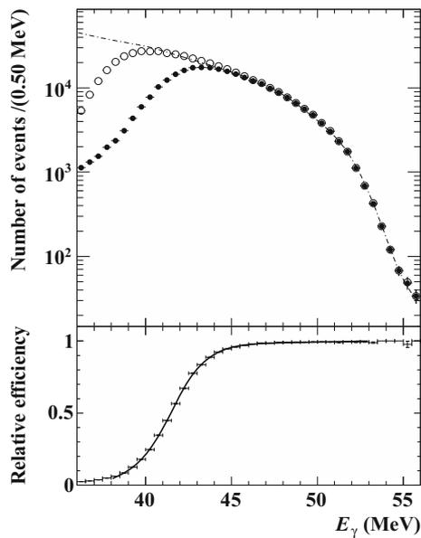
**Fig. 1** Photon energy spectra with different trigger thresholds (*top*). The *solid (open) circles* correspond to the normal (*lower*) threshold. The *dot-dashed line* is the MC simulation spectrum smeared with the detector response; the calculated spectrum is used to correct for the trigger effect in the lower threshold distribution. The *bottom plot* shows the ratio of the normal threshold spectrum to the lower threshold one
