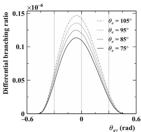
**Fig. 3** Differential branching ratio of RMD for  $P_{\mu^+} = -0.85$  as a function of  $\theta_{e\gamma}$  for four different values of positron polar angle  $\theta_e$ . These distributions are obtained by the numerical integration of Eq. (2) over  $E_e > 45$ ,  $E_\gamma > 40$  MeV, and  $\phi_{e\gamma}$
