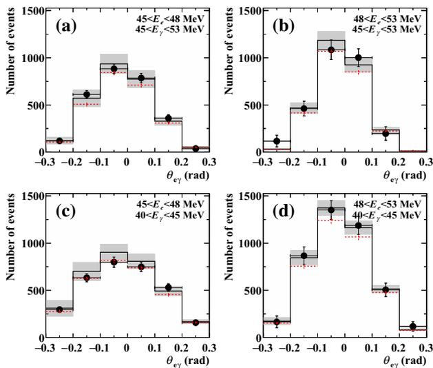
**Fig. 7** Distribution of RMD events in the 24 bins used in the fit. The *dots* show the data and the *solid lines* show the expected distribution with  $P_{\mu^+} = -0.85$  normalized by the Michel positron measurement. The *bands* show the systematic uncertainty (square root of the diagonal elements of the covariance matrix). The *red-dashed histograms* show the best-fit distribution
