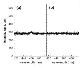
**Fig. 4** a The vertical scattering spectrum and b the horizontal scattering spectrum of the empty cell for 457.9 nm incident laser beam. The slit width was 1 mm and the integration time of the CCD was 20 s
