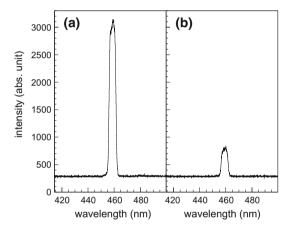
Fig. 5 a The vertical scattering spectrum and b the horizontal scattering spectrum of LAB for 457.9 nm incident laser beam. The slit width was 1 mm and the integration time of the CCD was  $20~\mathrm{s}$
