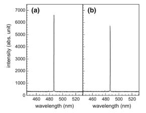
Fig. 3 a The vertical scattering spectrum and b the horizontal scattering spectrum of LAB for 488 nm incident laser beam. The slit width was 0.2 mm and the integration time of the CCD was 5 s
