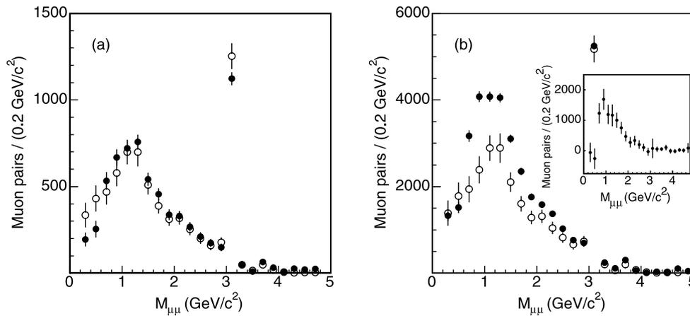
**Fig. 3** The invariant mass distribution of opposite-charge muon pairs in the data (●) is compared to the simulation prediction (○) for primary muons selected with (a) tight or (b) no SVX requirements. One of the two primary muons in the event is combined with an additional muon of opposite charge if their invariant mass is smaller than 5 GeV/c<sup>2</sup>.
