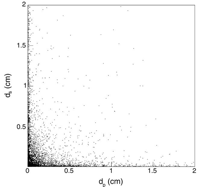
**Fig. 4** Two-dimensional distribution of the impact parameter of a primary muon,  $d_p$ , versus that,  $d_s$ , of additional muons in the ghost sample. All muons are selected with standard SVX requirements
