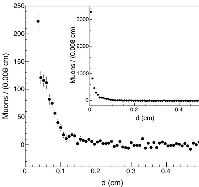
**Fig. 6** Magnified impact parameter distribution of additional muons in events in which both trigger muons satisfy the tight SVX selection. The fake muon contribution has been subtracted. The entire distribution is shown in the *insert*. Additional muons are selected without any SVX requirements
