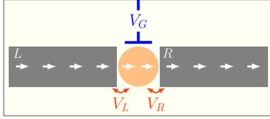
**Fig. 1.** Single-electron transistor. The quantum dot is asymmetrically coupled to the left ( $L$ ) and the right ( $R$ ) leads, with couplings  $V_L$  and  $V_R$ , respectively. The gate potential  $V_G$  controls the dot energy. The arrows indicate the direction of conduction.
