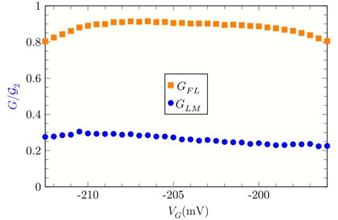
**Fig. 5.** Fixed-point conductances  $G_{LM}$  and  $G_{FL}$  as functions of the gate voltage  $V_G$ . At each gate voltage, the LM and FL fixed-point conductances result from extrapolating the  $G(T/T_K)$  vs.  $G_S(T/T_K)$  plots to  $G_S = 0$  and  $G_S = 1$ , respectively, as illustrated by each panel in Figure 4.
