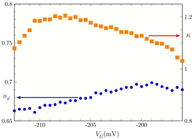
**Fig. 6.** Coupling asymmetry index  $\kappa$  and ground-state dot-level occupation  $n_d$  as functions of the gate voltage  $V_G$ . At each gate voltage, equation (41) determines  $\kappa$ , while equation (40) determines  $n_d$ .
