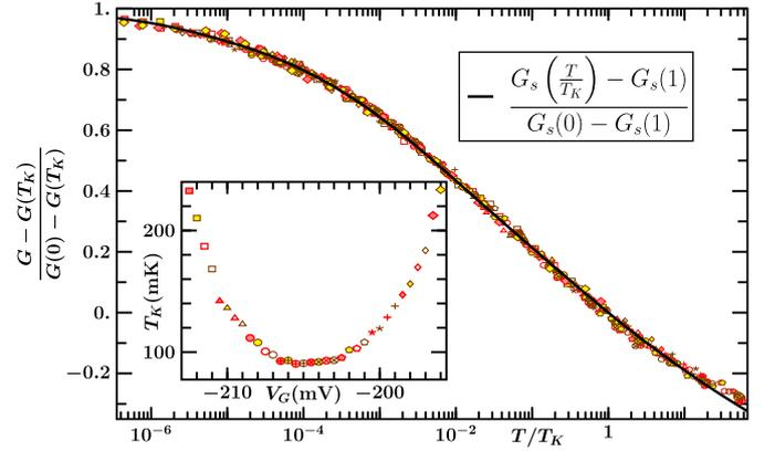
**Fig. 4.** Scaled zero-bias conductance  $G(T)$  (symbols) and universal function  $G_S(T/T_K)$  (solid line), as functions of  $T/T_K$ . Each symbol represents the former for one of the 34 gate voltages  $V_G$  in reference [22]. In the inset, the same symbol shows the corresponding  $T_K$ .
