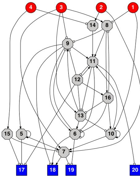
**Fig. 2.** Example of network. There are  $N_{in} = 4$  receptors (red circular nodes 1, 2, 3 and 4),  $M = 12$  middle nodes (gray octagons), and  $N_{out} = 4$  output nodes (blue square nodes 17, 18, 19 and 20). Connections ending in filled arrows are excitatory and connections ending on white empty squares are inhibitory.
