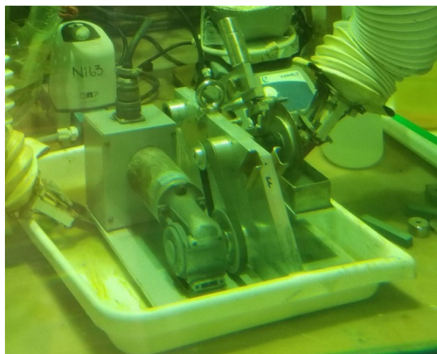
Fig. 4 Buehler IsoMet™ Low Speed Precision Cutter sawing the outer stainless-steel capsule of a californium source
