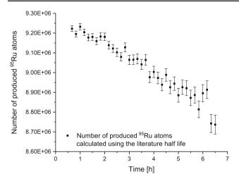
**Fig. 1** The number of  $^{95}Ru$  isotopes produced in the  $^{92}Mo(\alpha,n)^{95}Ru$  reaction as a function of time after the activation calculated from the 336.40 keV peak area using the literature half-life (t<sub>1/2</sub> = 1.643  $\pm$  0.013 h). The slope of the data indicates that the half-life value may be overestimated
