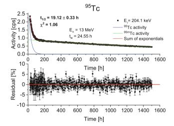
**Fig. 4** Decay curve (and residual) obtained from the measured  $E_{\gamma} = 204.1 \, \text{keV} \, \gamma$ -transition of  $^{95}\text{Tc}$ . The width of each time bin is 2 h before and 4 h after 188.00 h long counting
