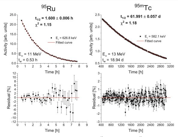
Fig. 3 Decay curves (and residuals) based on the study of the  $E_{\gamma}=626.8\,\text{keV}$  ( $^{95}$ Ru) and  $E_{\gamma}=582.1\,\text{keV}$  ( $^{95m}$ Tc)  $\gamma$ -transitions. The widths of each time bin are 10 min for  $^{95}$ Ru and 12 h for  $^{95m}$ Tc
