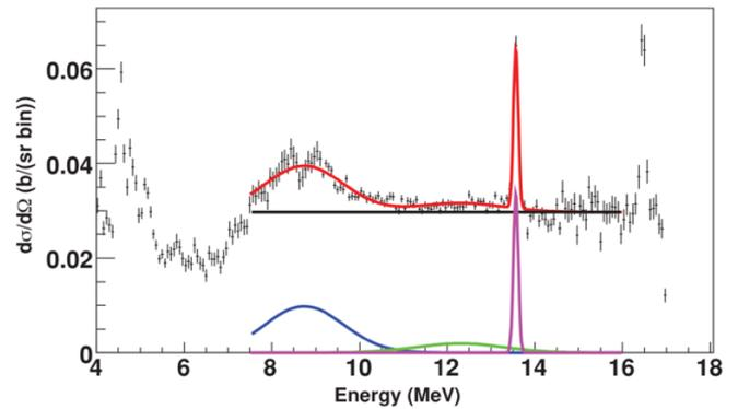
**Fig. 3.** (Color online) Excitation energy spectrum of  $^{118}\text{Sn}$  for the 0 degree measurement at  $E_p = 50$  MeV. The individual fits for a linear background (black), deep-hole states (blue), a possible GPV around 12 MeV (green), and oxygen contaminant (magenta) are shown together with the total fitting function (red). The bin width is 67 keV/bin. From ref. [13].
