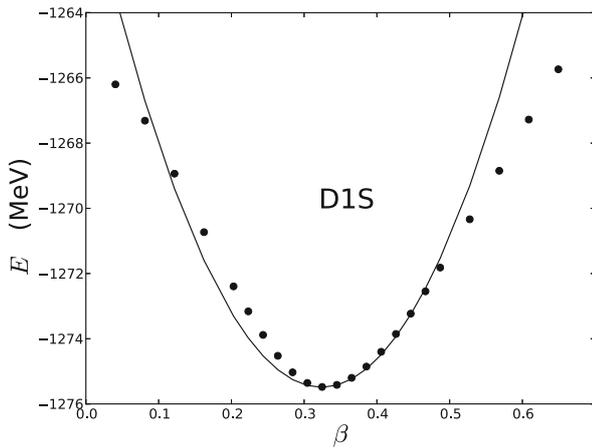
**Fig. 2.**  $^{156}\text{Gd}$  energy as a function of  $\beta$  in self-consistent mean field theory, shown as filled circles. The line is a fit to a quadratic dependence on  $\beta$ , eq. (14). The  $k$  parameter of the fit is  $k = 298$  MeV,  $225$  MeV, and  $337$  MeV for the D1S, BCPM, and SLy4 functionals, respectively.
