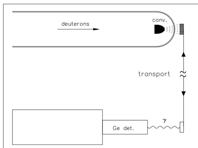
**Fig. 1.** Schematic layout of the experiment, not on scale. The neutrons generated in the converter target activate either the foils used to measure the neutron spectrum or react with  $^{18}\text{O}$  in the water target to produce  $^{15}\text{C}$ . For a detailed description, see ref. [9].
