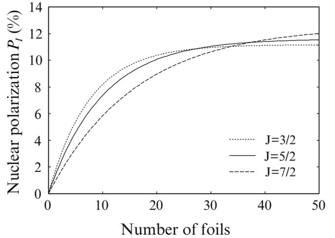
**Fig. 1.** Calculated nuclear polarization as a function of the number of the foils by using eq. (1) with the atomic polarization of 3%. Here, the dotted, solid and dashed lines were calculated using the averaged atomic spin  $J = 3/2$ ,  $5/2$  and  $7/2$ , respectively.
