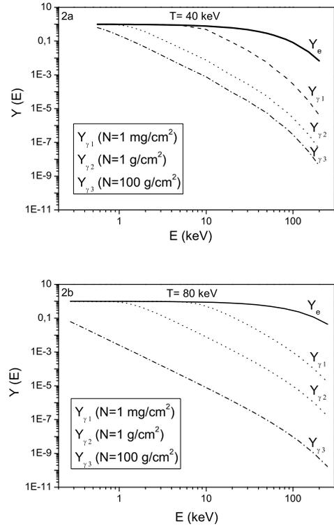
**Fig. 2.** The REC photon spectra due to the electron capture in the plasma clouds for electrons with  $T = 40$  keV (top) and  $T = 80$  keV (bottom) and for the column densities varying between  $1 \text{ mg/cm}^2$  and  $100 \text{ g/cm}^2$  (or between  $1.5 \times 10^{21}$  and  $1.5 \times 10^{26} \text{ atoms/cm}^2$ ).
