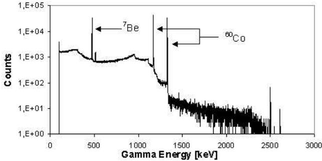
Fig. 2. Gamma spectrum of Pd sample measured in Naples ( $\Delta t = 1$  h).
