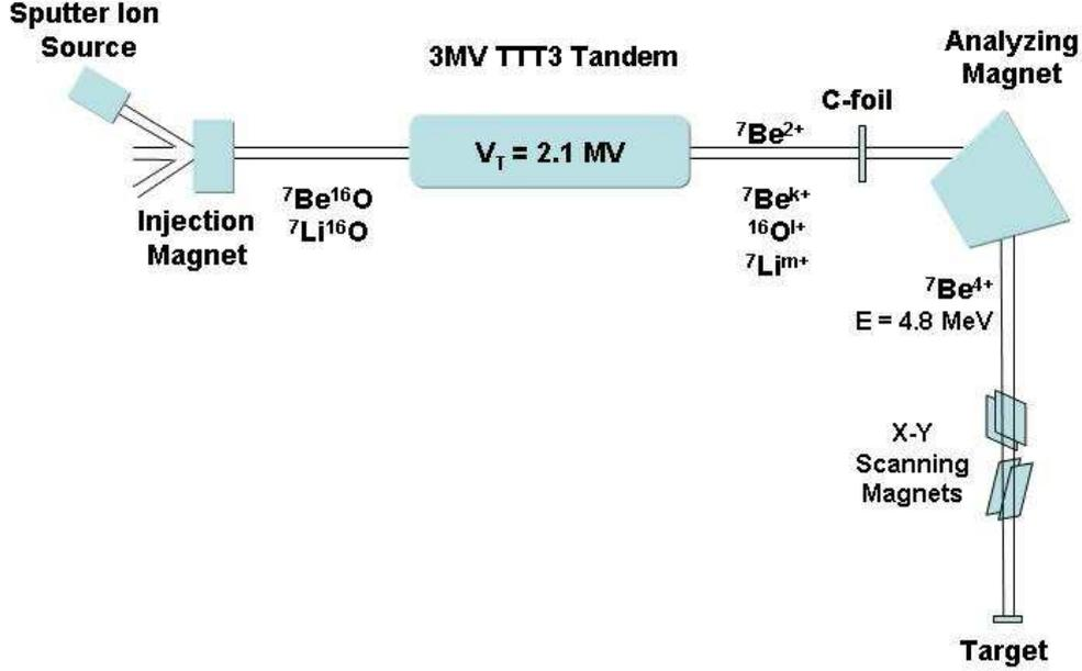
Fig. 1. Scheme of the  ${}^7\text{Be}$  implantation setup at the TTT3 Tandem accelerator of the Federico II University of Naples.
