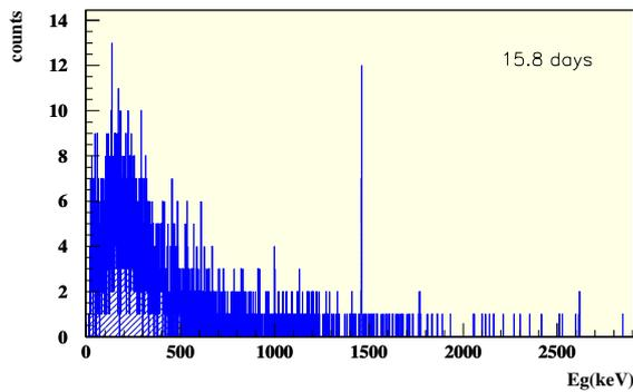
**Fig. 4.** Background  $\gamma$ -ray spectrum obtained with the ultra-low background 125% HpGe detector at the low activity laboratory at LNGS. The measuring life-time is 15.8 days.
