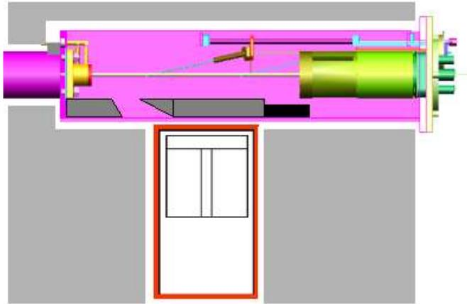
**Fig. 3.** Schematic view of the inner part of the target chamber. The internal lead collimator, the beam power calorimeter, the movable setup for the silicon detector and the long collimator before the carbon foil (at  $20^\circ$  with respect to the beam direction) are shown. The HpGe detector is positioned below the target chamber.
