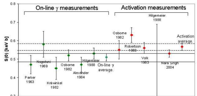
**Fig. 1.** Summary of past measurements performed with the on-line  $\gamma$  detection technique and the activation method. With the new activation measurement by Nara Singh *et al.* [4] the discrepancy between the two methods is reduced from 15% to 11%.
