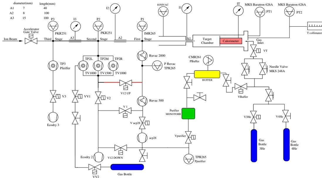
**Fig. 2.** Schematic diagram of the windowless gas target system.
