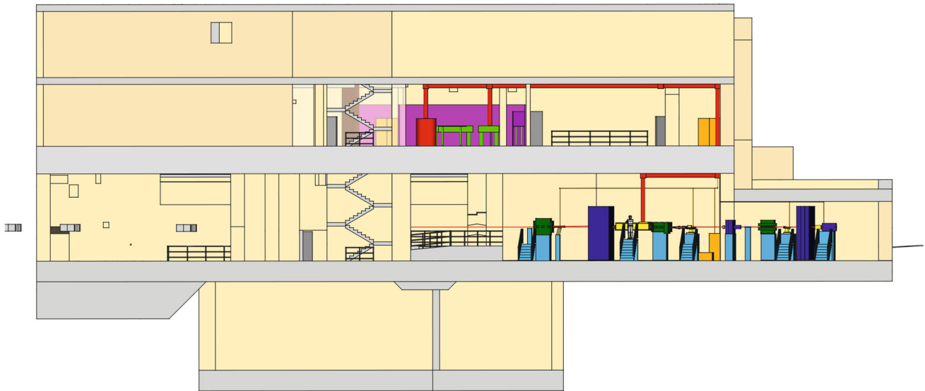
Fig. 97 Side-view CAD drawing of the XS1 access shaft building, including the LUXE experiment. The building is shown in beige and grey, while the different experimental elements are shown coloured. The laser clean room is shown in magenta, the laser and electron beam pipes are shown in red, the supporting structure are shown in light blue, the magnets are shown in green, the shielding and dumps are shown in dark blue, the different active components (interaction chambers (IC), and detectors) are shown in yellow, and the services are shown in orange
