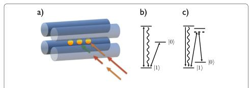
**Figure 1 Quantum simulations with trapped ions. (a)** Scheme of a rf Paul trap for digital-analog quantum simulations. Energy-level scheme for optical qubits (**b**), and rf qubits (**c**). In addition to the qubit levels |0⟩ and |1⟩, a third level is used for qubit readout.
