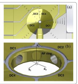
It is well known that Maxwell's equations forbid the possibility to use a static electric field to trap charged particles in free space through Earnshaw's theorem. However, a static electric field can create a saddle-point, which confines the charged particles in some directions and deconfines them in the other directions. A static electric field that provides a saddle-point is
