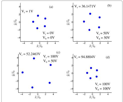
Figure 6 Equilibrium positions (blue dots) for N=5 with various DC voltages on the RF ring and independently applied to the top and bottom electrodes. The equilibrium shape remains the same for the four cases shown: (a)  $V_t = 1 \text{ V}$  and  $V_t = V_b = 0 \text{ V}$ , (b)  $V_r = 36.147 \text{ V}$  and  $V_t = V_b = 50 \text{ V}$ , (c)  $V_r = 52.225 \text{ V}$ ,  $V_t = 100 \text{ V}$ , and  $V_b = 50 \text{ V}$  and (d)  $V_t = 94.880 \text{ V}$  and  $V_t = V_b = 100 \text{ V}$ .
