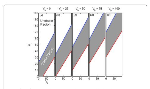
Figure 4  $\beta_1$  and  $\beta_3$  are both real when the ion configuration is stable (shaded grey). We use Eq. (14) to find a region where the ion configuration is stable. The white regions are unstable.
