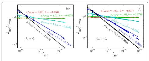
Figure 8 Spin-spin coupling versus distance for different detunings with DC voltages of  $V_r = 94.9 \text{ V}$  and  $V_t = V_b = 100 \text{ V}$  and different number of ions (different panels; (a) is N = 10 and (b) is N = 20) on a log-log plot. The colored lines are the fit to a power-law behavior  $J_{mn} \propto r_{mn}^{-b}$ . The detunings are  $\mu = 1.001, 1.01, 1.1, 2$ , and 11 to the blue of  $\omega_{CM}$  in units of  $\omega_{CM}$ .
