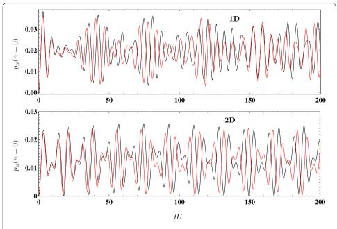
**Figure 3 Numerical solutions for small lattices.** Probability to have no particles on a lattice site in one-dimensional lattice of 11 sites (1D) and for two-dimensional lattice of 3 × 3 sites (2D). Red lines - exact diagonalization (the same as in Figure 2), black lines - numerical solution of Eqs. (6), (8).
