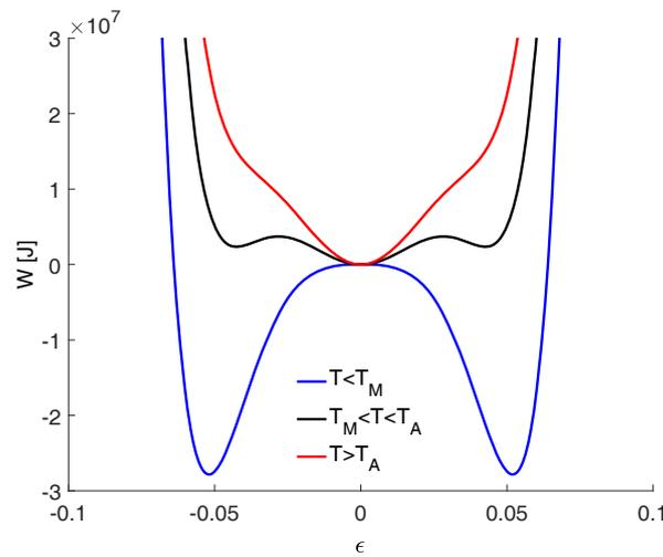
**Fig. 4.** Free energy of SMA spring at different temperatures according to Falk's model.
