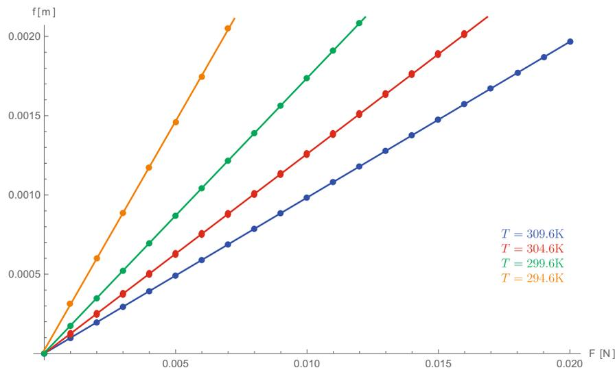
**Fig. 7.** Stiffness characteristics of shape memory CMA for different ambient temperatures.
