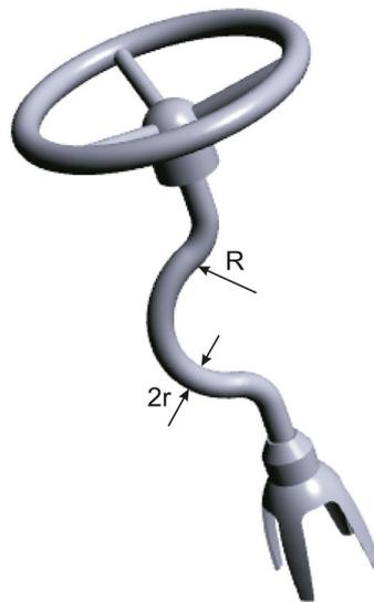
**Fig. 3.** Conceptual view of the C-shape memory prosthesis of the middle ear made of SMA.
