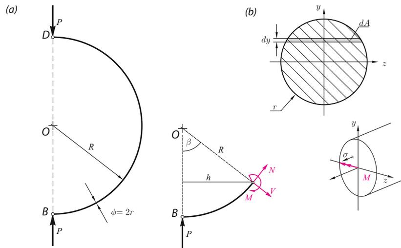
Fig. 5. Analytical model of the half-ring middle ear system prosthesis.
