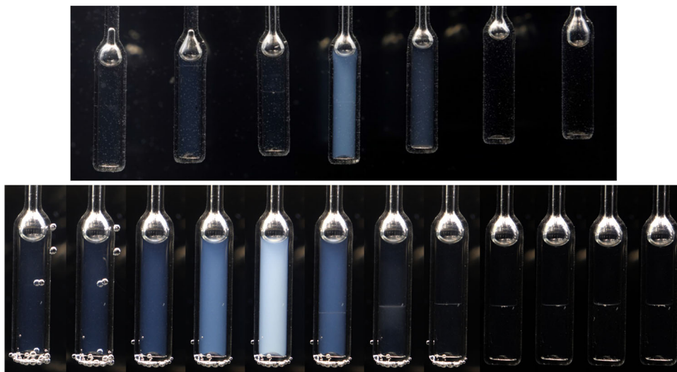
Fig. 2 Upper photograph of 3-picoline—deuterium oxide mixtures in the surrounding of the critical concentration, near the critical temperature. The white-bluish critical opalescence, signaling the vicinity of the critical point, is visible. Lower image is a collection of single ampule photographs with lowering temperature (from left to right) depicting opalescence onset (milky white color near the critical temperature) then clearly visible meniscus and its slight movement
