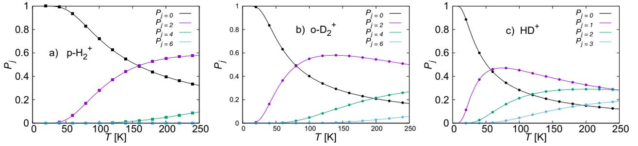
**Fig. 6.** Steady-state solution of the rate equations for  $p\text{-H}_2^+$ ,  $o\text{-D}_2^+$  and  $\text{HD}^+$  as a function of collisional temperature. In this calculations we do not include the spontaneous downward relaxation rates of  $\text{HD}^+$ . Continuous lines are the computed solutions using a SVD technique. The points correspond to the Boltzmann distribution.
