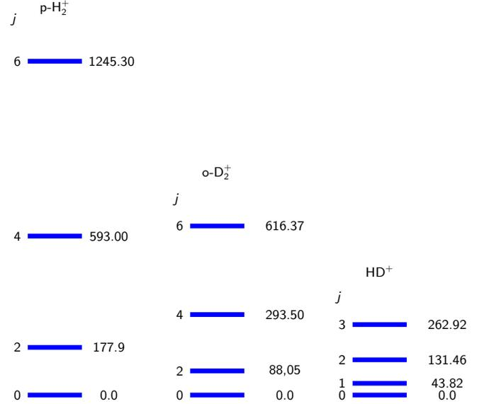
**Fig. 3.** Rotational energies (in  $\text{cm}^{-1}$ ) for the first four rotational levels of all three molecules discussed in the present work. All levels are given within the pseudo- $^1\Sigma$  reduced coupling scheme (see main text for details). The rotational constants employed are:  $29.65 \text{ cm}^{-1}$  for  $\text{H}_2^+$ ,  $14.675 \text{ cm}^{-1}$  for  $\text{D}_2^+$  and  $21.91 \text{ cm}^{-1}$  for  $\text{HD}^+$ .
