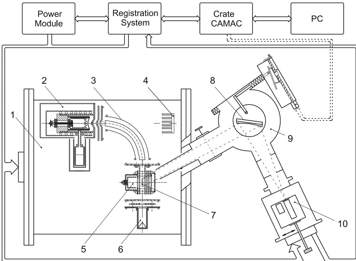
**Fig. 1.** Schematic layout of experimental setup: 1 – vacuum chamber, 2 – ion source, 3 – electrostatic ion selector, 4 – cooled atom trap, 5 and 6 – deep Faraday cups, 7 – electron gun, 8 – diffraction grating, 9 – vacuum monochromator, 10 – cooled solar-blind photomultiplier.
