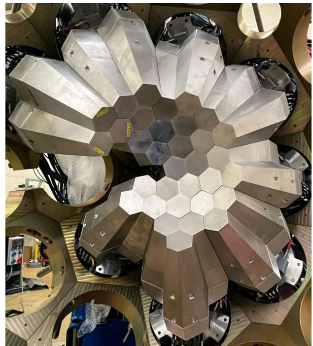
Fig. 20 The array with 11 triple detector modules during commissioning of the spectrometer at LNL in 2022
