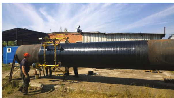
Fig. 9. Conduct of the bench adhesion tests at the testing ground of OOO Delan.
