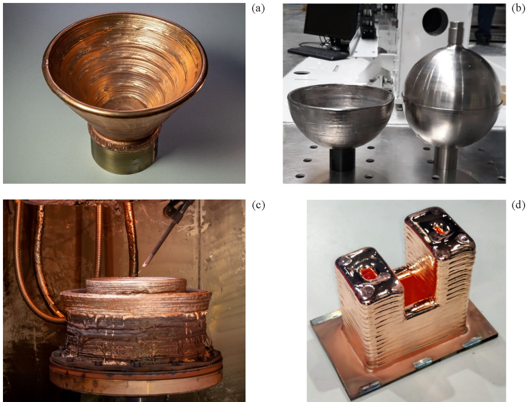
Fig. 1. Large-sized products for the aerospace, metallurgical and electrical applications fabricated by the EBAM method from bronze (a), titanium alloy (b), copper (c, d): a—as-built rocket thrust chamber liner; b—as-built part (left) and spherical tank made of two parts (right); c—as-built blast furnace tuyere nose; d—as-built part electrical brush gear holder (color online).
