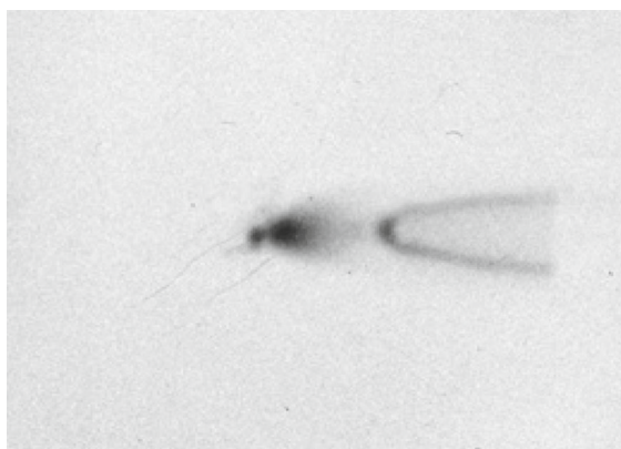
Fig. 2. X-ray obscurogram of the interelectrode gap recorded under the following conditions: at the time of the discharge initiation, the internal electrode is the anode, the outer electrode is the cathode, and the length of the forming line is 1 m.
