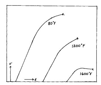
Fig. 2— e - r data for Pt 8W alloy at various temperatures
