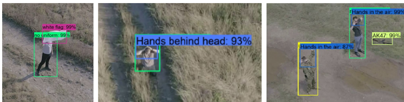
Fig. 3 Highly-magnified examples of classifier detecting and classification as part of a video stream: (i) a person without uniform with a white flag, (ii) non-uniformed person with hands behind their head,
