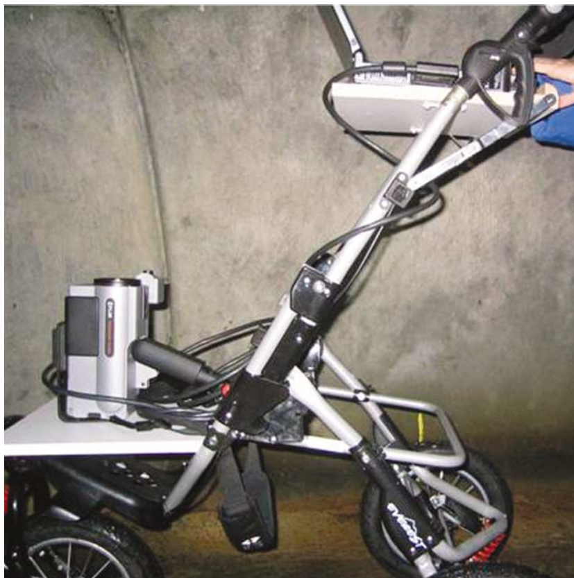
Figure 6: Infrared thermography measurement device
