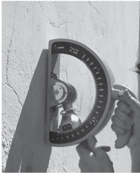
Figure 11: Pendular Schmidt impact hammer test.
