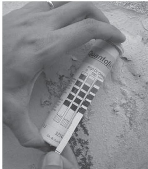
Figure 10: Strip tests – semi-quantitative determination of salts.
