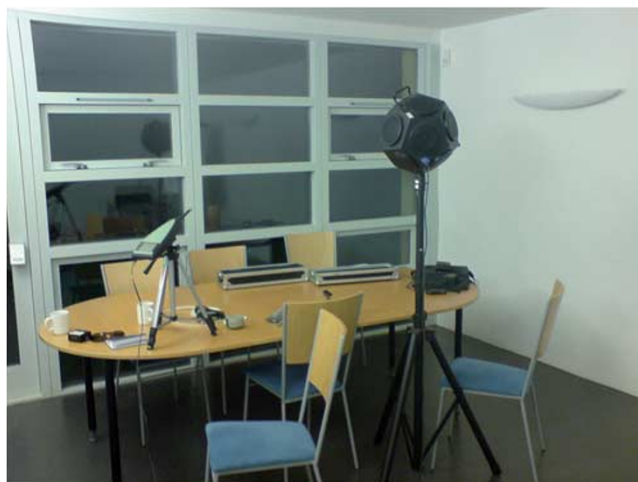
Figure 1: The audio analyser and the omni-power sound source.
