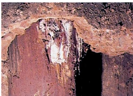
Figure 9: Top of a pole from a pile foundation showing attack by the polefungus Physisporinus vitreus
