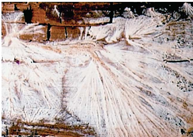
Figure 8: Fan-shaped strandmycelium of the mine polypore Antrodia vaillantii on the surface of decayed timber showing a brown rot
