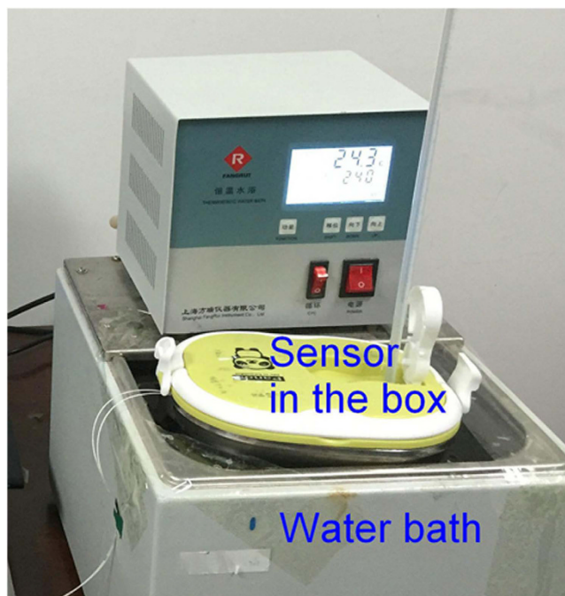
Figure 4. Experiment setup for temperature sensitivity measurement.
