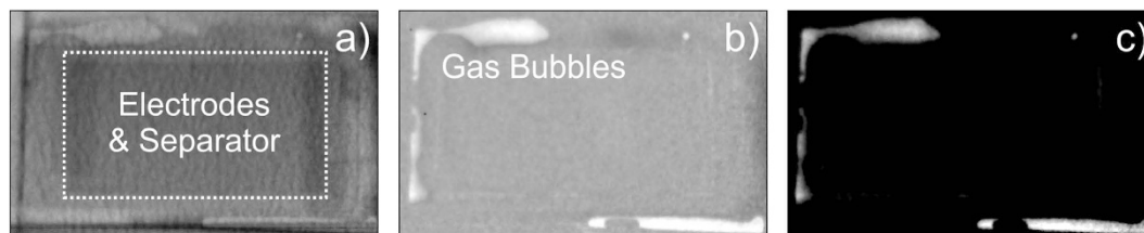
Figure 1. Neutron transmission images of a pouch cell illustrating the different processing steps. (a) After noise reduction, (b) after normalization to the first image, and (c) after segmentation, with grey areas representing the generated gas.
