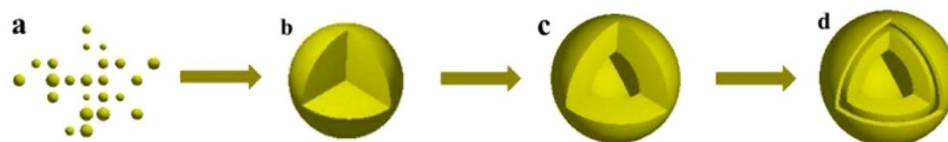
Figure 5 | Schematic exhibition of the formation of double-shell CoO hollow particles.
