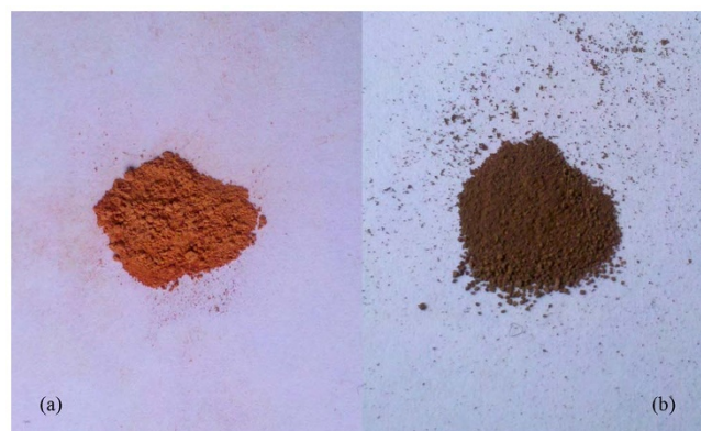
Figure 3 | The pictures of products prepared by microplasma in different electrolyte: (a) \text{H}_2\text{O} –ethylene glycol (1 : 1) and (b) pure distilled water.
