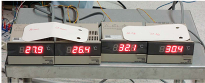
Figure 3 The body surface temperature measuring devices (SENTECH) were used in the experiment. The two devices on the left indicate the body surface temperature of the upper extremities, and the other two on the right indicate the body surface temperature of the lower extremities.
