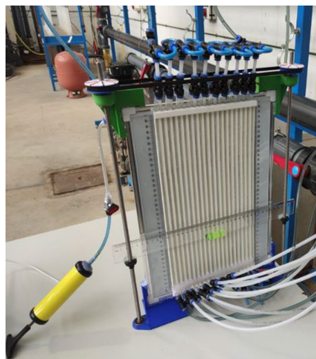
Figure 3. Bank of piezometric tubes to measure the pressure head differences.
