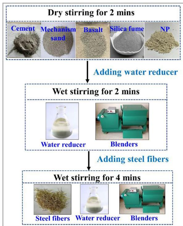
**Figure 3.** Mixing process of ultra-high-performance concrete.
