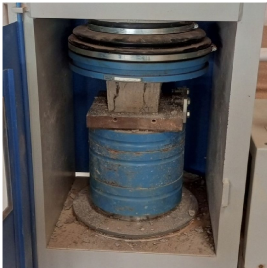
Figure 3. Specimen failed under compressive strength test.
