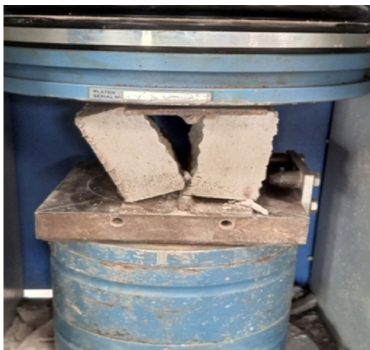
Figure 4. Split block specimen under tensile strength test.
