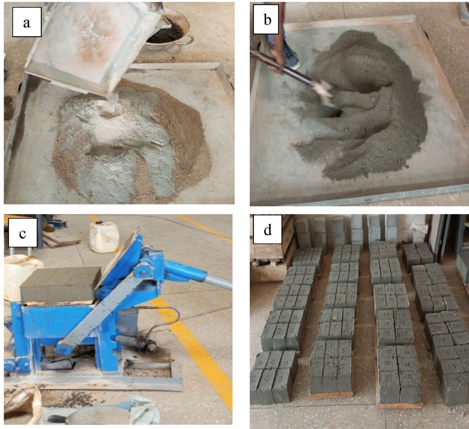
Figure 2. Production process of sancrete block specimens: (a) spreading of cement and CAA on the sand, (b) mixing of the materials, (c) moulding of the block specimens using compressed block making machine, (d) curing of the block specimens.
