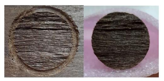
**Figure 7.** Pull-off specimen of the thermally-modified beech substrate illustrating full and accepted failure in the body of the wood substrate (no failure occurred in the adhesive layer) (magnification  $\times$  2.5).
