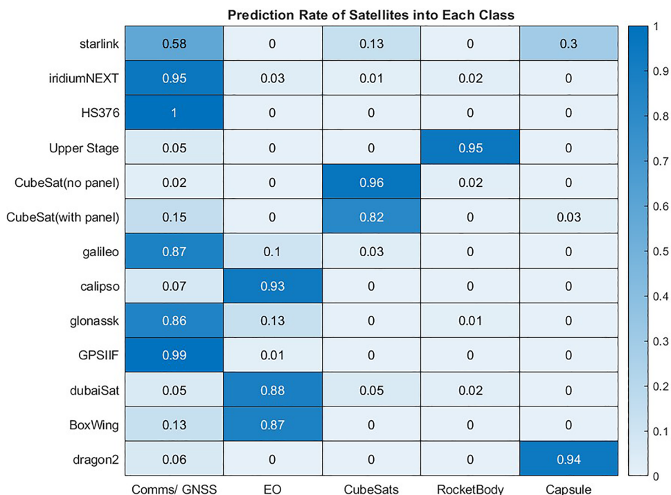
Figure 26. Prediction rate from the knn model when classifying objects based on probability of materials present on the object.
