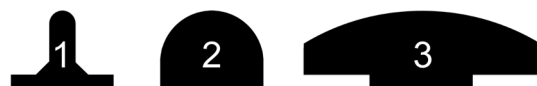
Figure 5. Considered terrain shapes with circular shapes of 10 mm (1), 40 mm (2), and 160 mm (3) in radius.
