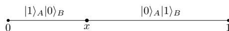
Figure 2. Brownian motion on a line of unit length, where a particle starts at position x . The probability of the particle reaching endpoint 1 is x , while the probability of the particle reaching endpoint 0 is 1 - x .
