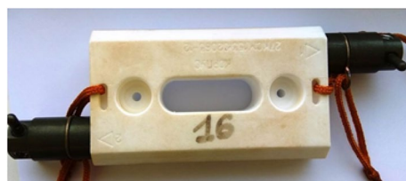
Figure 1. Photo of the "Test" transport module with the rods installed after 2 exposure years.
