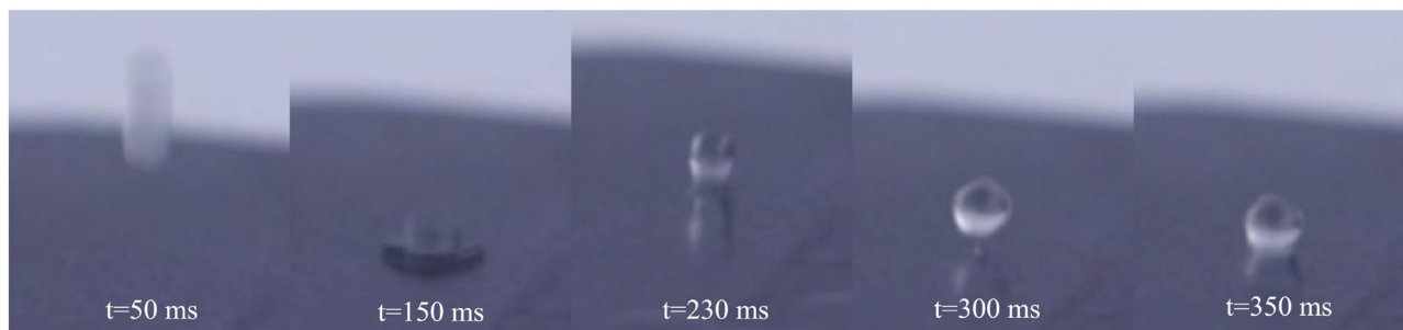
Figure 4. The surface of T-shaped reentrant nanostructured PFOTS/Si surface displayed the bouncing of hexadecane droplets as captured by a sequence of high-speed digital camera photograph.
