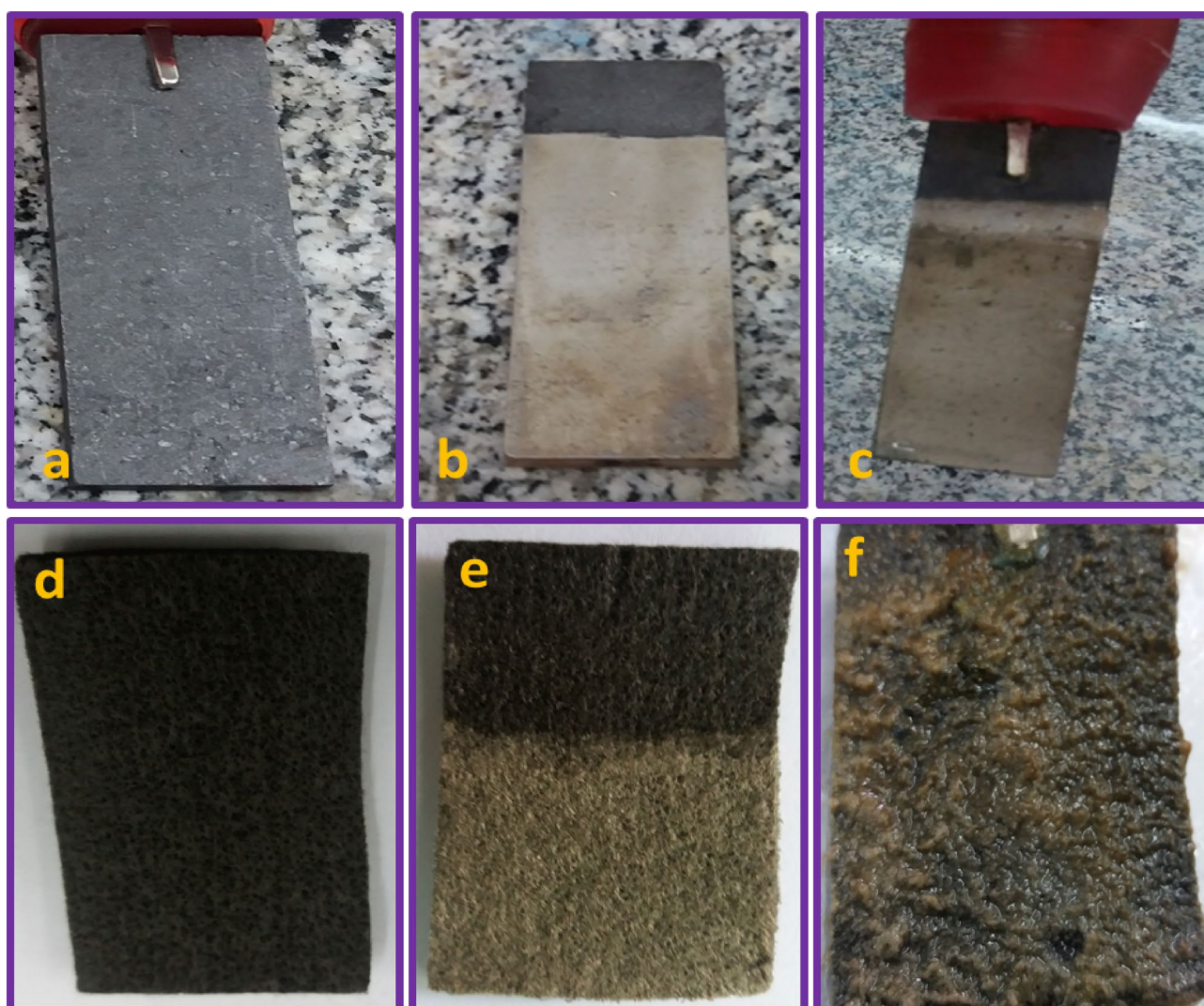
Figure 9. Real photographic images of the (a,d) bare GP and CF; (b,e) Ni@CF and Ni@CF; and (c,f) bio-Ni@CF and bio-Ni@CF electrodes.
