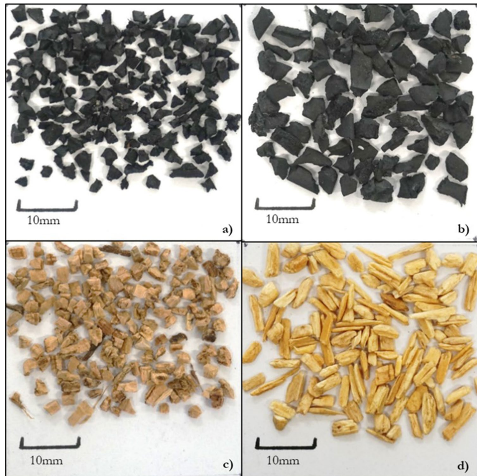
Figure 2. The performance infills used in the study, (a) SBR, (b) Recycled EPDM, (c) Cork, (d) Pine woodchip.
