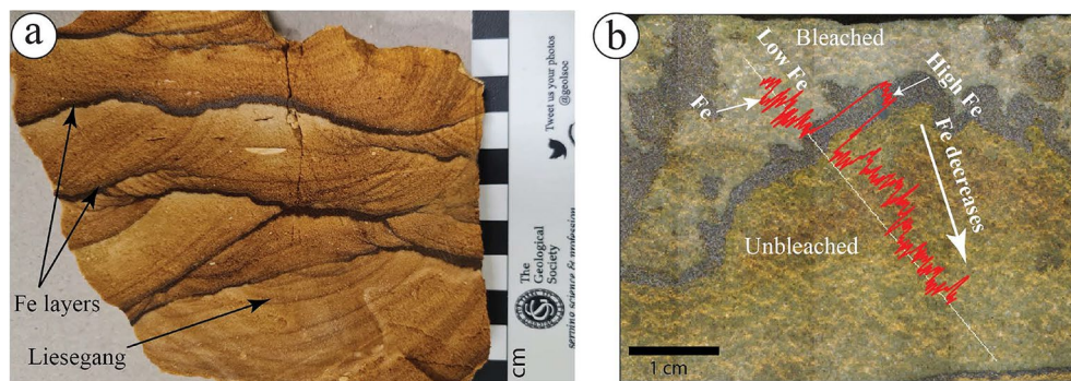
Figure 21. The distribution of (a) ferruginous (Fe) layers and liesegang bands, and (b) Fe distribution within Fe layers and associated unbleached and bleached areas. Note that Fe layers show a higher concentration of Fe that decreases gradually in the unbleached area and becomes almost absent in the bleached area.
